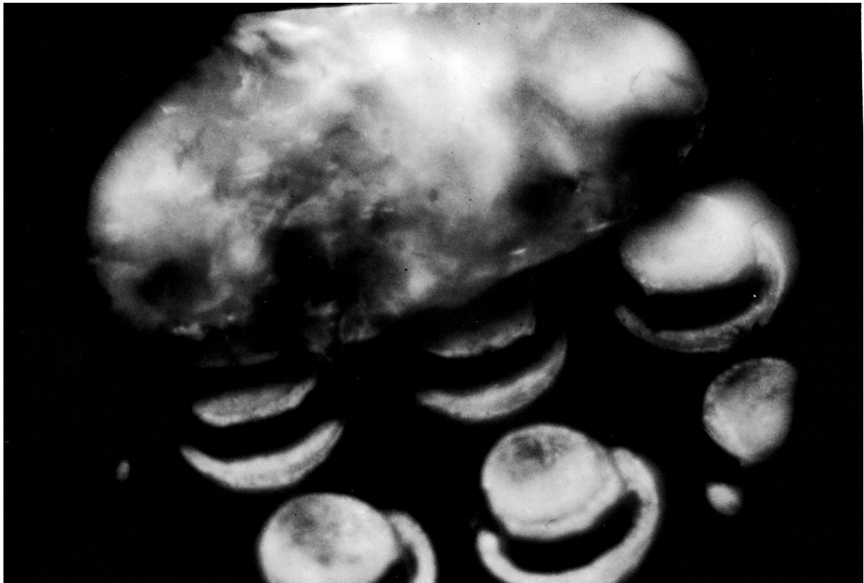
Figure 80. Edge of Ethanol Drop on Cylindrical Pins
